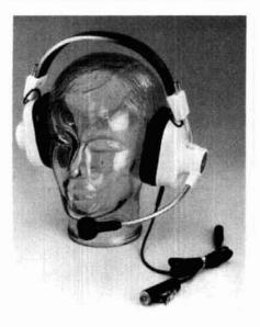
SET/MIC was developed to permit improved transmission and reception with the TR-720 in noisy environments. This new accessory is light (12 ounces) and features cushioned, noise-attenuating ear pads that can be adjusted for a comfortable fit. A flexible boom supports and electret noise-cancelling microphone. Supplied with a 5-foot cable to connect to the radio, the unit comes with a push-to-talk switch attached. The CS-65 HEADSET/MIC lists for \$69.95.
